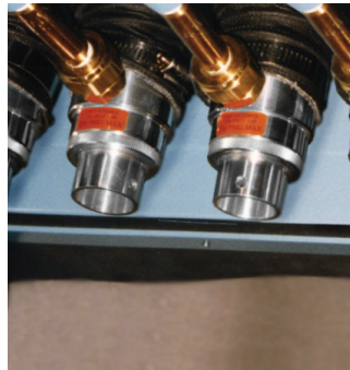
Adjustable Air Amplifiers are ducted to draw clean air for drying.
