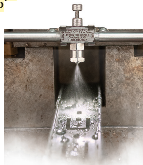
Model EF8010SS applies lubricant to a drawer slide.
