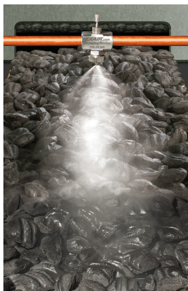
A Model AW1030SS is used to keep dust down during charcoal briquette production.
