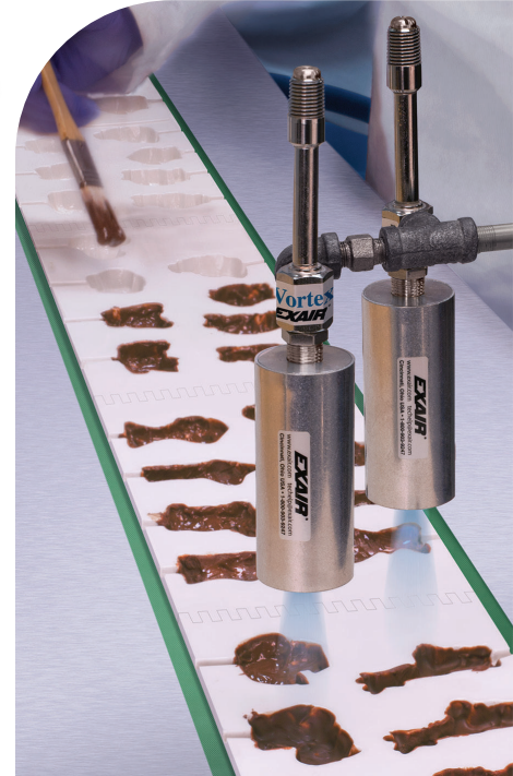
Dual Vortex Tubes rapidly cooling milk chocolate on a production line.
